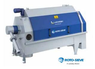
In addition to septic receiving, the Lackeby Roto-Sieve® septic unit RSS 36, is also suitable for storm flow and overflow screening.
