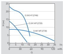
D = Solids-handling impeller.
