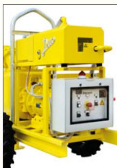
**Control panel with automatic star/delta starter as standard equipment**
