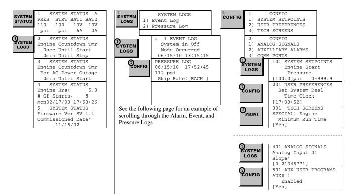
**<u>SYSTEM LOGS</u>**: The FD4 has three separate data logs; 1) alarm log, 2) event log, and 3) pressure log. The alarm log is a subset of the event log and only displays the last ten alarms that have occurred or cleared. The event log records all alarm and system function type events
