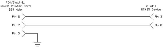
Modbus Setup From Controller Interface:
