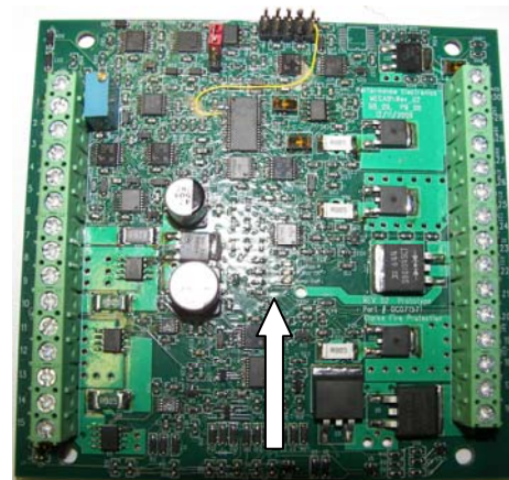
Figure #30 – MECAB speed switch
