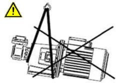
Never lift the pump at one suspension point only. Incorrect lifting may result in personal injury and/or damage to property.
