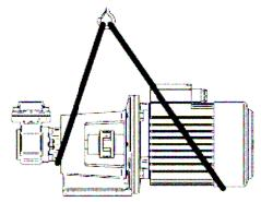
Always use two ropes to be secured in such a way that the pump cannot slip. Make sure that the pump unit is suspended in a horizontal position! !
