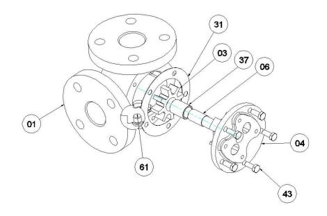
Remove the screws (43). Where present, use the two threaded bores to facilitate removal. When removing the cover (04) make sure that the seal (31) will not be damaged. If damaged, replace it.
