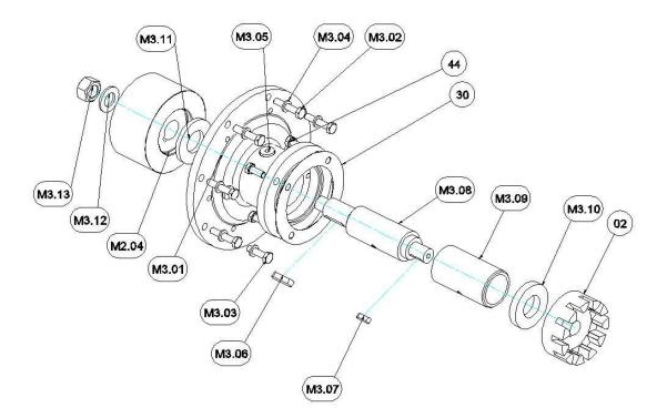
Unscrew the screws (44) and pull-off the casing (01).
