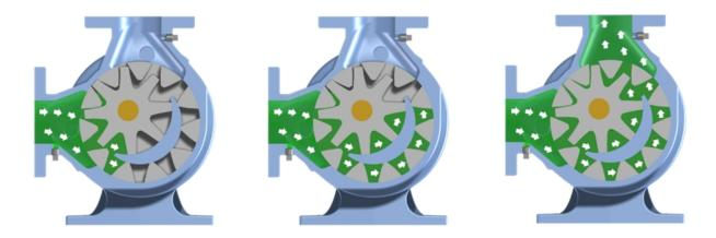
The figure above shows the liquid as it advances through the pump; the point where the teeth come out of mesh governs the phase of the liquid entering between the rotors and is, therefore, physically located close to the suction zone. The liquid is carried between the teeth and the steady and the discharge opening developing as the teeth come into mesh eject the liquid.
