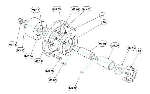
Unscrew the bolts (M3.02) and (M3.03) and pull-off the complete plug-in unit from the bearing bracket (M1.01).
