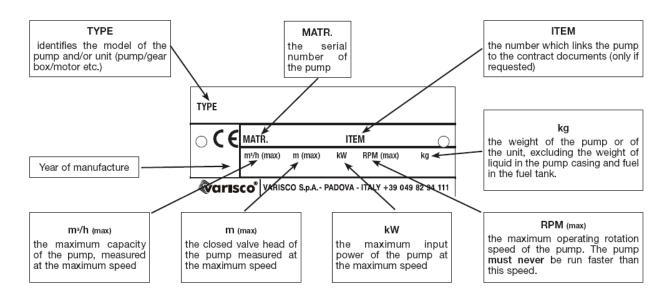
The data on the nameplate relates to a final acceptance with oil at 20℃ and a viscosity of 100 cSt.
