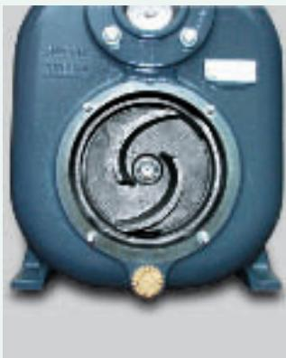
► Balanced ductile iron or stainless steel two blade impeller handling solids up to 3" in diameter. Pump out vanes on rear to reduce the build up of foreign matter and reduce the pressure on the mechanical seal.
