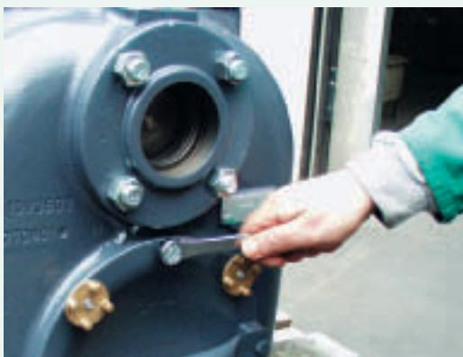
► Impeller inspection cover with large handle, brass wrenches and pusher bolts for easy removal.
