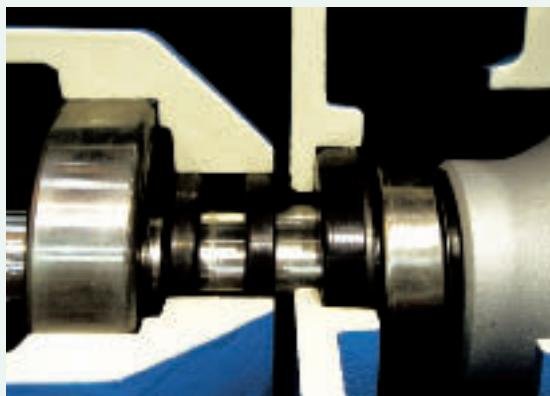
► Self-aligning mechanical seal with tungsten carbide faces and Viton® elastomers. Oil lubrication with double lip seal and cavity to isolate the seal oil from the bearing oil and permit monitoring of leaks from the seal from the outside.
