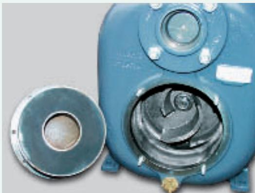
► Replaceable front and rear wear plates with abrasion and oil resistant rubber facing (except for ST-R8). The rubber facing protects the impeller blades against wear due to small abrasive particles, reducing the need for adjustment to take up wear, thus ensuring as new performance and priming well into the service life of the wear parts. Cast iron and stainless steel wear plates available on request.
