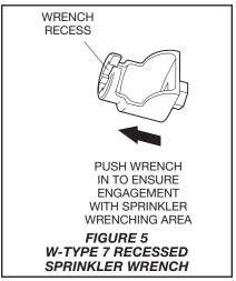
sprinkler, loosen the wrench jaws before removing the wrench.
