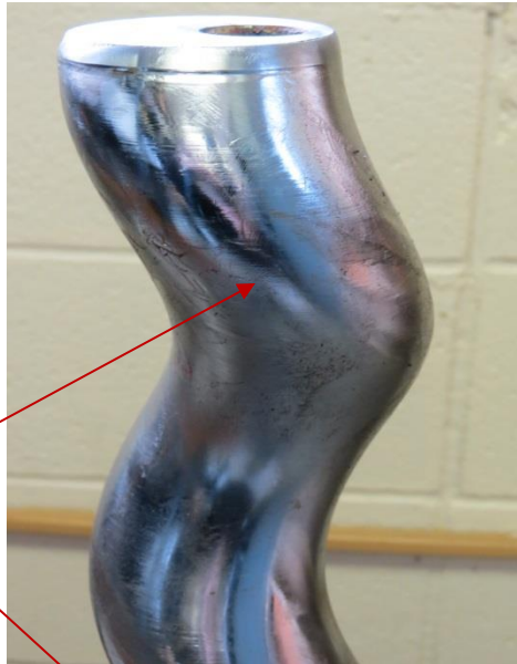
Parts have even wear patterns
