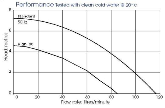
NOTE: These magnetically coupled pumps are designed for use with clean fluids. Solids will cause jamming. Abrasives will reduce pump life & invalidate the warranty. NEMP pumps are not self priming & are not designed to run dry The company reserves the right to change specifications
